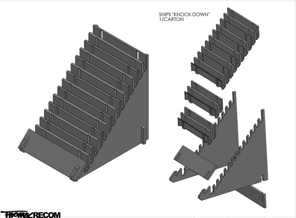
ESEARCH COMPANY INC. DESC.: 14 LEVEL "KNOCK-DOWN" CHANNEL DISPLAY PART#: 969M DATE: 6-24-19 SHEET 2 OF 3
