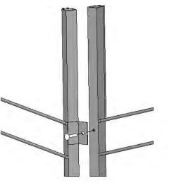
**4.)** DROP SIGNS INTO CHANNELS AND INSTALL PRONGS AS SHOWN HERE
